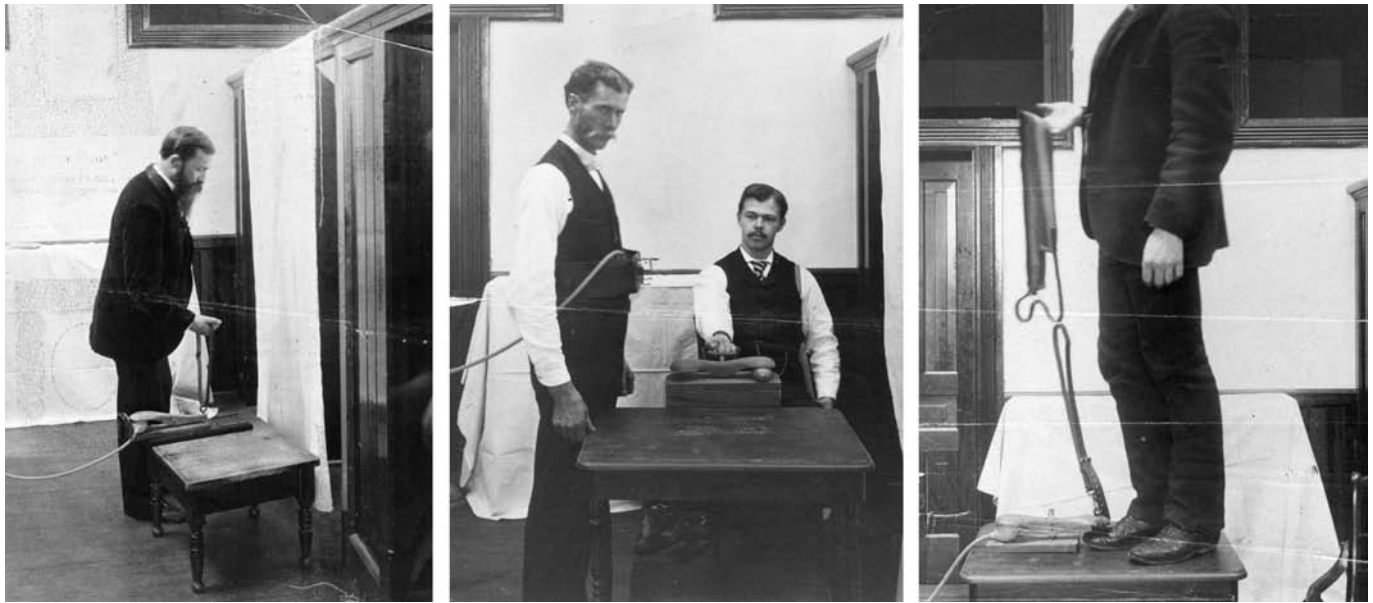
FIGURE I.25 • Kellogg's Universal Dynamometer acquired by Dr. Hitchcock to test the muscular strength of Amherst College students. From 1897 to 1900, strength measurements were taken on 328 freshmen, 111 sophomores, and 88 seniors, including retests of 58 individuals. Arm strength was measured bilaterally for the forearms and for the latissimus dorsi, deltoid, pectoral, and shoulder "retractor" muscles. Trunk measurements included the anterior trunk, and anterior and posterior neck. The leg measurements included the leg extensors and flexors and thigh adductors. (Left) "Arm pull." (Center) Anterior trunk (standing) and forearm supinators (sitting). (Right) Legs. (Photos courtesy of Amherst College Archives and by permission of the trustees of Amherst College, 1995.)
