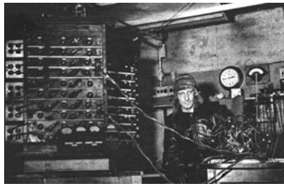
FIGURE I.28 • In 1944, researcher Donald Griffin tests the equipment he designed to assess heat distribution in gloves at -40^{\circ}\text{F} . (From Folk, GE. The Harvard Fatigue Laboratory; contributions to World War II. Adv Physiol Educ 2010;34:119.) ( www.advancedphysiology.org/content/34/3/119.full.pdf+html )
